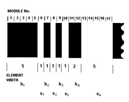
Figure 22 - PDF417 is composed of 4 elements whose widths add up to 17 modules
