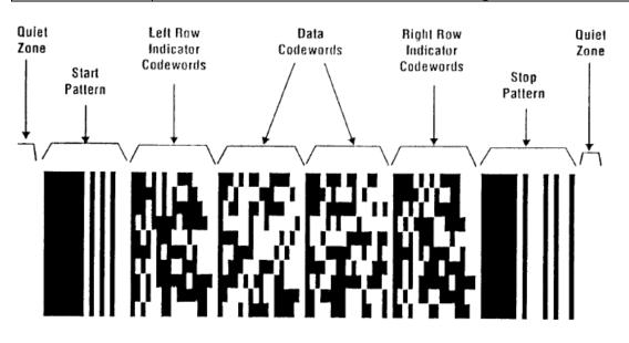
Figure 21 - Structure of the PDF417 symbol as defined in the ISO/IEC 15438
