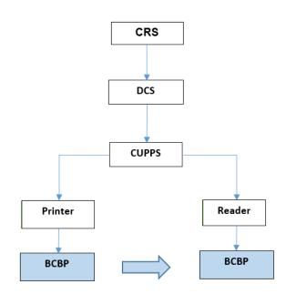
Figure 9 - Data flow in a CUPPS environment
