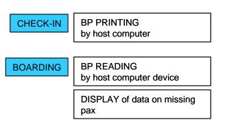
In the Automated Boarding Control process (Recommended Practice 1789), as the host computer prints the boarding pass at check-in and reads it at boarding, it can display the list of missing passengers. Or, if the reader is stand-alone, it can display a list of sequence numbers boarded to identify missing passengers, and the agent can then use the DCS interface to obtain data on missing passengers.
