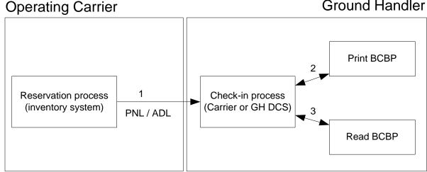
Figure 6 - Data flow of passenger information at check-in
